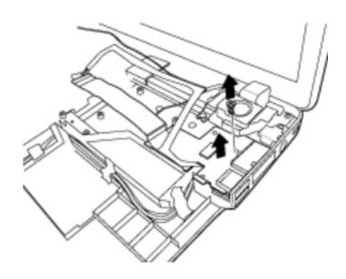
Figure 4-31 Removing screw securing LAN board
